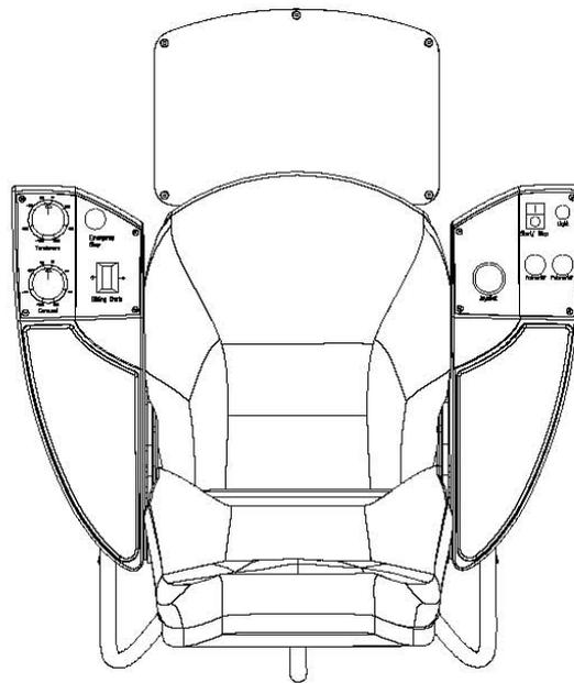
Controls of the Cable Handling Equipment arranged in the Operator's Chair
